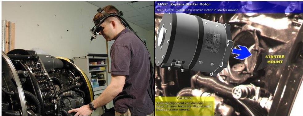
Figure 2: Instructional overlays in the Augmented Reality for Maintenance and Repair (ARMAR) system. Photo used with permission of S. Henderson, Columbia University Graphics and User Interfaces Lab.
